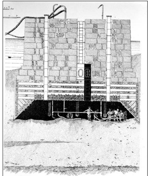
Fig. 9. Pneumatic bridge caisson, Blair Crossing Bridge over the Missouri River near Blair, Nebraska, c. 1883, George S. Morison, designer (George S. Morison, *The Blair Crossing Bridge*, 1886, as reproduced in Ira O. Baker, *A Treatise on Masonry Construction*, 8th ed. New York: John Wiley and Sons, 1897. Library of Congress, Prints and Photographs Division, *Historic American Engineering Record*, HAER NEB, 89-BLAIR.V, 1-4).
