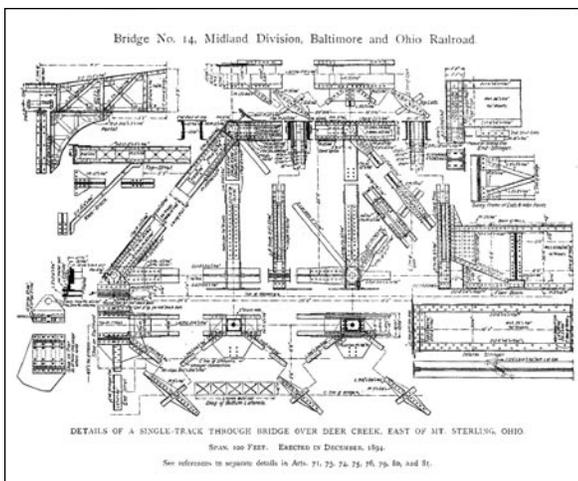
Fig. 8. Pin-connected railroad bridge over Deer Creek, east of Mount Sterling, Ohio, 1894, Baltimore and Ohio Railroad, designer (Mansfield Merriman and Henry S. Jacoby, *A Text-Book on Roofs and Bridges*, Part III, Bridge Design, 4th ed. New York: John Wiley and Sons, 1905, Plate III).
